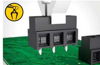
Automated assembly process using gripper or vacuum system
